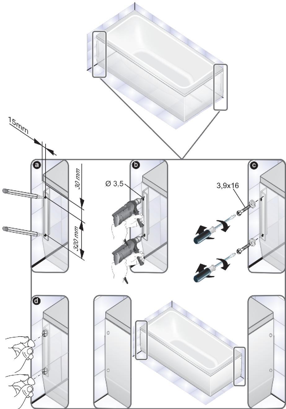
**INSTALACIÓN FALDÓN FRONTAL - LATERAL DERECHO / INSTALLATION OF FRONT - SIDE RIGHT PANEL / INSTALLATION DE TABLIER FRONTAL - LATÉRAL DROIT**
